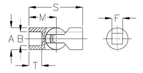
$\begin{array}{lll} A & = 80 \\ F & = 42 \\ M & = 115.0 \\ Max torque (Nm) = 930 \\ s & = 230 \\ T & = 58 \end{array}$
